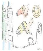
er open flame as they will heat the pipe too quickly and may cause it to explode!) Some people recommend wrapping rags over a frozen pipe and pouring boiling water over it. Obviously, this method is very messy! Never pour boiling water directly onto a frozen pipe.
